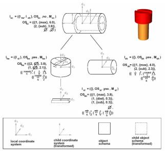
Figure 4: Example of an IDT representation for a stylized screw.
