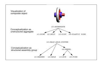
Figure 6: Assembly conceptualization
