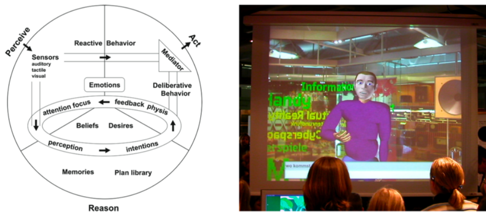
Figure 3.5: Left: MAX's cognitive architecture [70]. Right: MAX acting as a museum guide [62], p. 2.
