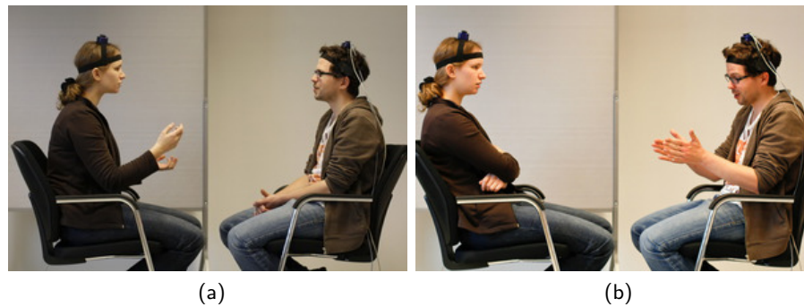
Figure 4.8.: Data acquisition in an animal guessing task. Both interacting participants are wearing a head-mounted motion sensor and are taking turns in guessing the animal the other is thinking of. Pictures taken by Christian Leichsenring.
