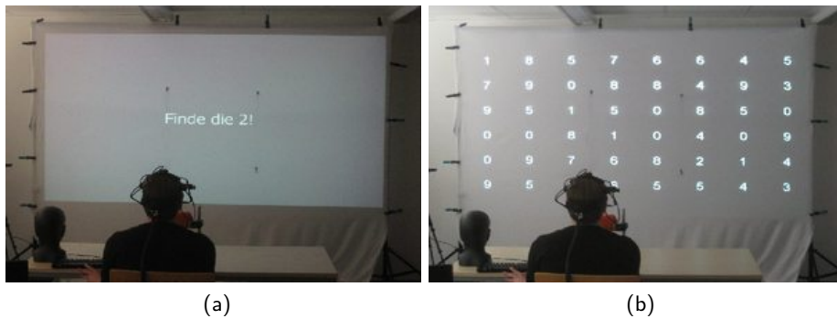
Figure 4.7.: Stimuli presentation for the visual search scenario: (a) search target “Find the 2!”, (b) number grid
