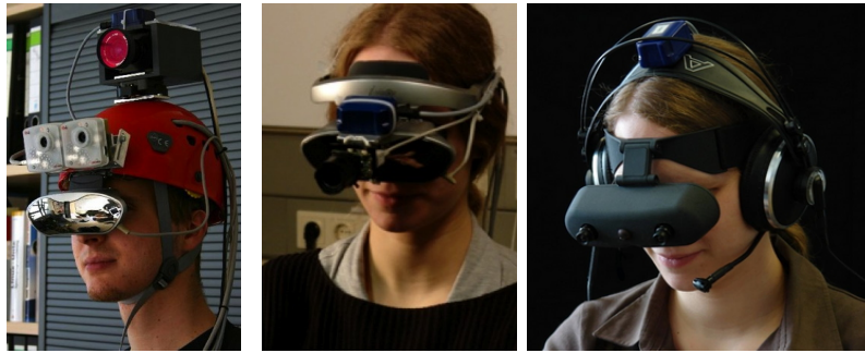
Figure 5.2.: Hardware improvements. The HMD hardware was reduced and improved in weight and user comfort over the past years and extended to use a set of sensors. left: oldest version, right: version used in this thesis.
