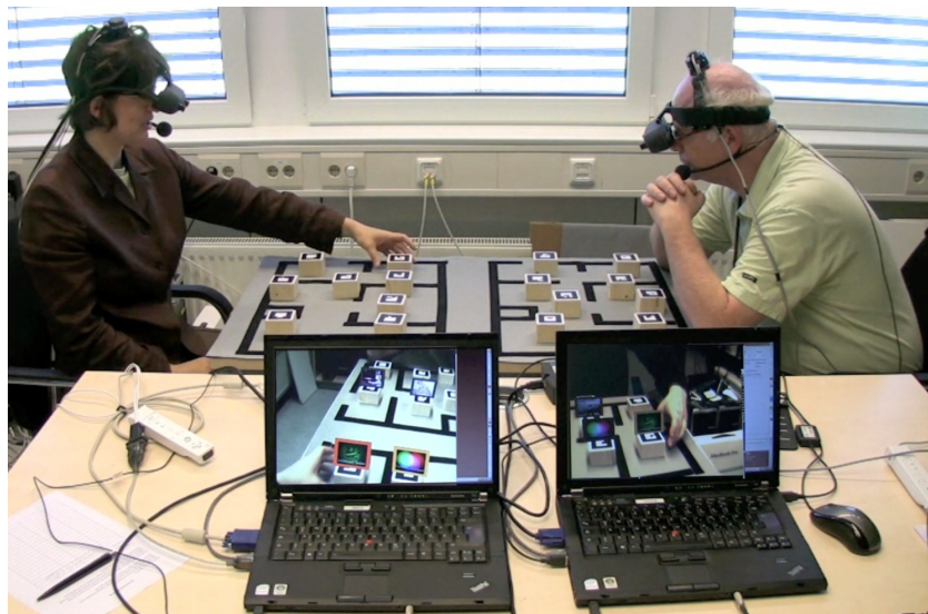
Figure 4.6.: The interactive exhibition design scenario: Two participants are positioning interactive exhibits in a museum plan. The computer screens show (enlarged) the participant's current view through the AR goggles.
