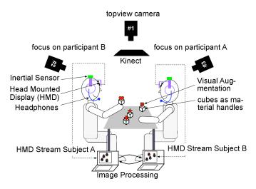
Figure 1: The schematic shows the setup and the hardware components that ARbInI aggregates. These include static components such as three DV cameras, a Microsoft Kinect and two to three workstations for data processing. Each participant wears a headmounted display, a microphone headset and a BRIX motion sensor to measure head movement at high temporal resolution.
