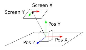
Figure 4: Marker Tracking allows us to retrieve the objects position (in cm) and screen position (in pixel) for every used symbol. Pos Y represents the height above ground and is used to identity whether an object is placed on the table or lifted. Object movement results in changes to Pos X and Pos Z. The screen is identical to the observers point of view which makes the screen position a good feature to adapt parameters according to that perspective.
