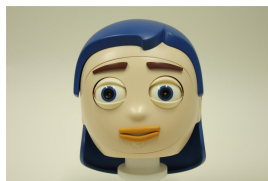
Fig. 1. Anthropomorphic robot head Flobi
