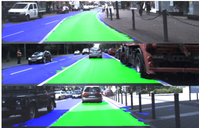
Figure 3.5.: Exemplary inner-city scenes of the road terrain detection with marked ego-lane (green) and road area (blue). In the visualization, the blue road area is occluded by the green ego-lane.
