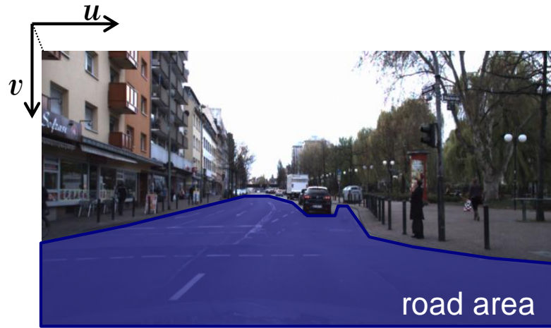
Figure 4.8.: Ground truth for road area: image regions are labeled using polygons. In the perspective image positive samples for road area, i.e., the region within the polygon, are colored blue.
