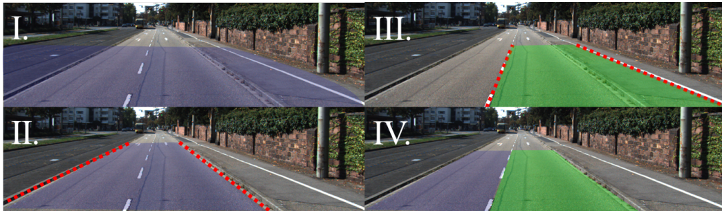
Figure 3.1.: Road terrain detection in urban areas for road area (blue) and ego-lane (green). (I) depicts an example result of a surface-based approach using the height over ground as feature. In (II), a curbstone-based road area detection approach is demonstrated. (III) represents the result of a lane marking based ego-lane extraction. In (IV), the desired result with a separation of the ego-lane from the road area is depicted.
