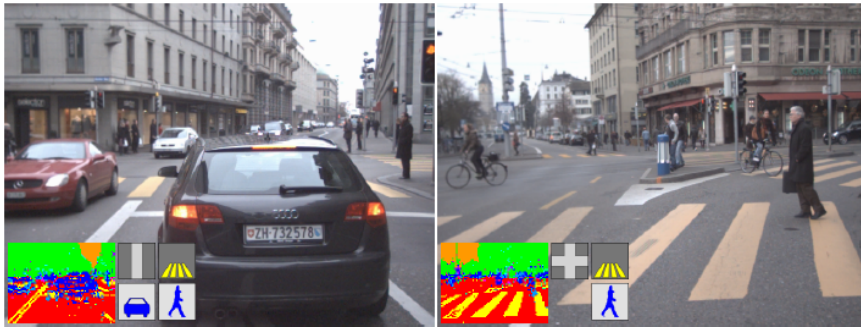
Figure 2.1.: Traffic scene understanding by classifying the scene category. Estimation is based on holistic segmentation of the image (bigger box on the lower left), inference of scene category is denoted by the darker and the existence of pedestrians and cars with the brighter small gray boxes. Pictures are extracted from Ess et al. (2009).
