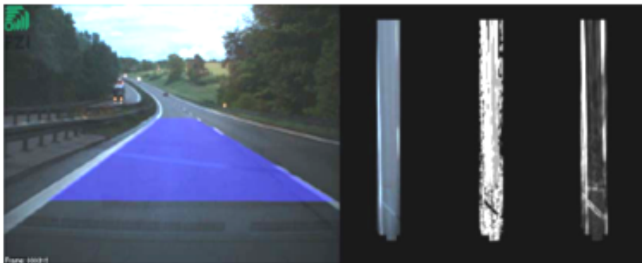
Figure 2.8.: Visual features extracted from the ego-lane surface (see blue region in left part) are analyzed in the Birds Eye View (right part). Picture is extracted from Gumpp et al. (2011) .
