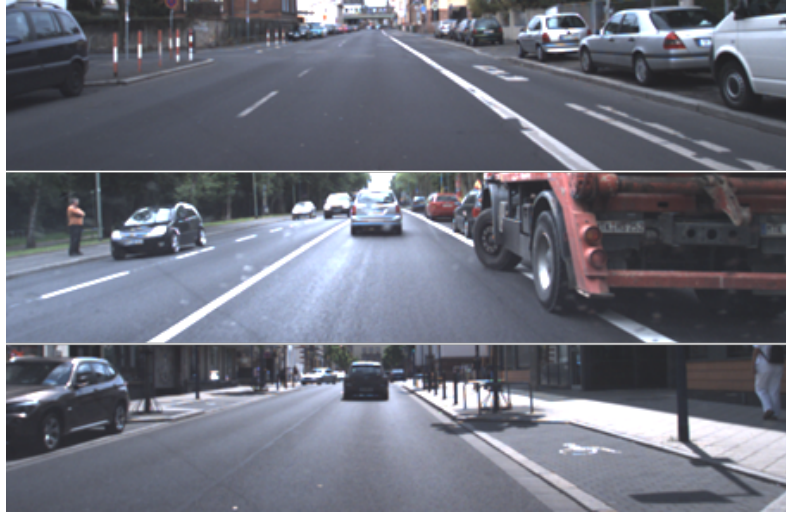
Figure 1.5.: Challenging scenarios in urban areas: Bad lane marking qualities, occlusion of road delimiters, flat curbstones and unmarked roads.
