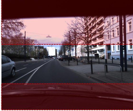
Figure 4.1.: Input image of the LVA-system captured by an in-car mounted camera. The colored part denotes regions that are cropped before processing.
