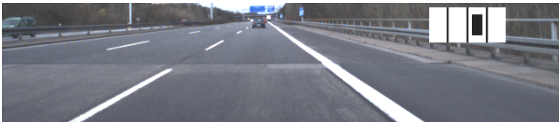
Figure 6.2.: Demo image showing a typical scene on a German highway. Here the left ego-lane index is 2, and the right ego-lane index is 1.
