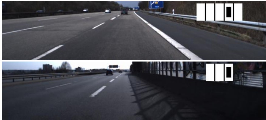
Figure 6.5.: Exemplary classification results where estimated ego-lane indexes are illustrated with white boxes. The black box denotes the ego-lane.
