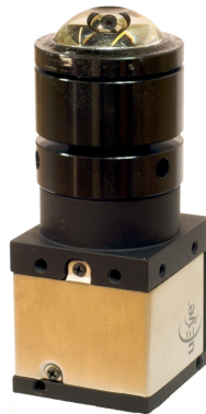
(2) Catadioptric setup with panoramic annular lens. H: 8 cm, \varnothing : 3 cm, FoV: -17^\circ/38^\circ . Camera: IDS uEye UI-2220-M [D8], PAL: Tateyama PAL-S25G3817-27C [D16].
