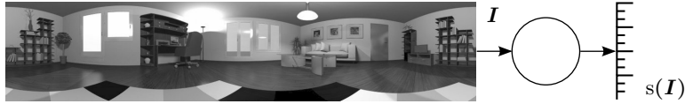
Figure 3.11.: Signature-based place representation. Places are characterized by low-dimensional global signatures s = s(I) derived from the entire omnidirectional image I .
