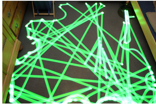
(2) Random walk obtained by the iRobot Roomba 770. The robot was released from its docking station (top right) and returned to it after 689 s. The thick green trace results from the robot's control elements.
