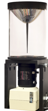
(3) Catadioptric setup with hyperbolic mirror. H: 20 cm, \varnothing : 7 cm, FoV: -90^\circ/46^\circ . Camera: ImagingSource DFK4303 [D11], lens: Pentax TS2V314A [D5], mirror: Accowle Large Type Wide Angle [D1].
