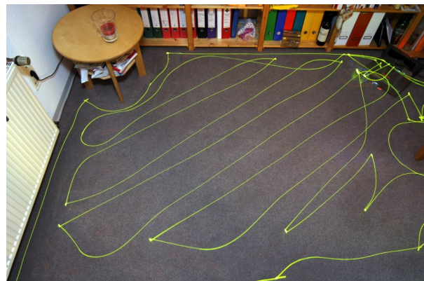
(2) Neato XV-11. The robot was released from its charging station (top right) and successfully returned to it after 448 s.
