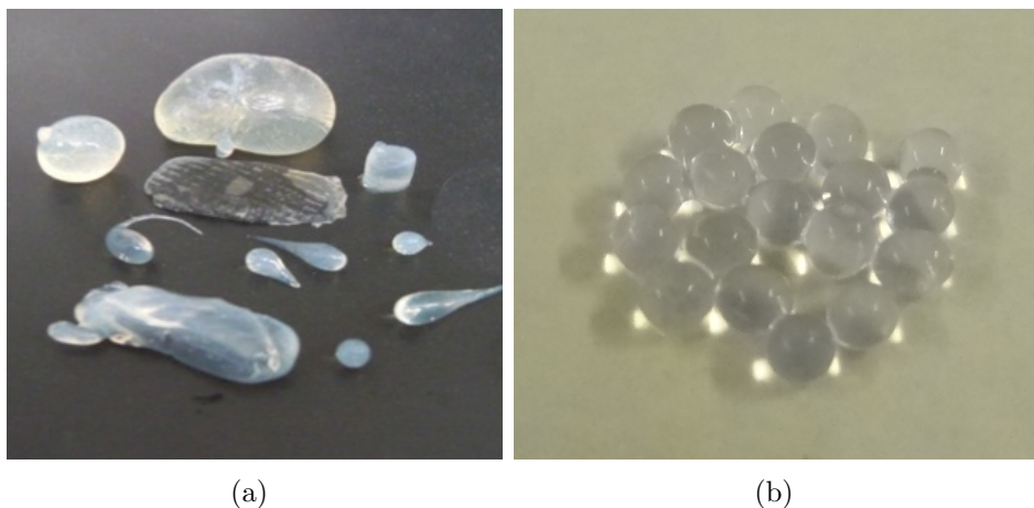
Figure 3.11: Different shapes have been formed from alginate gel (a). Spheres with an diameter of about 3 mm were fabricated by dropping alginate solution in the curing agent (b).
