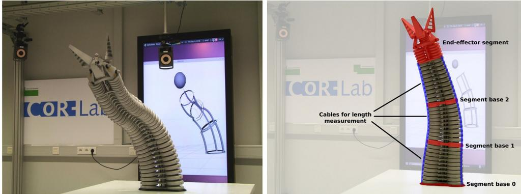
Fig. 6.1: The bionic handling assistant (BHA) (left). The segments and respective length sensors of the BHA (right).
