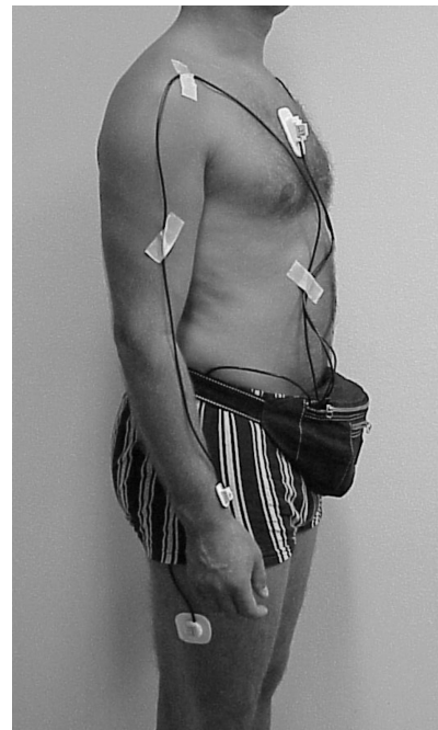
Figure 3.5.: The activity recognition system with wired accelerometers as used in the publication of Bussmann et al. [17]
