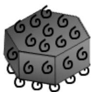
Figure 95: Different possibilities of peptide adsorption. Top: c25-mms6 only adsorbs onto the (111) crystal face. Bottom: The synthetic polypeptide adsorbs onto all crystal faces.
