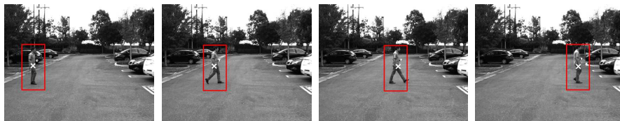
Figure 1.5: Example of pedestrian detection using camera images and pattern recognition. Reproduced with permission from [35].
