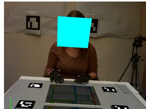
Figure 3: Overlay of the virtual representation over the scene camera image of the eye tracking device. The position of the participant’s face is calculated by a face detection algorithm.
