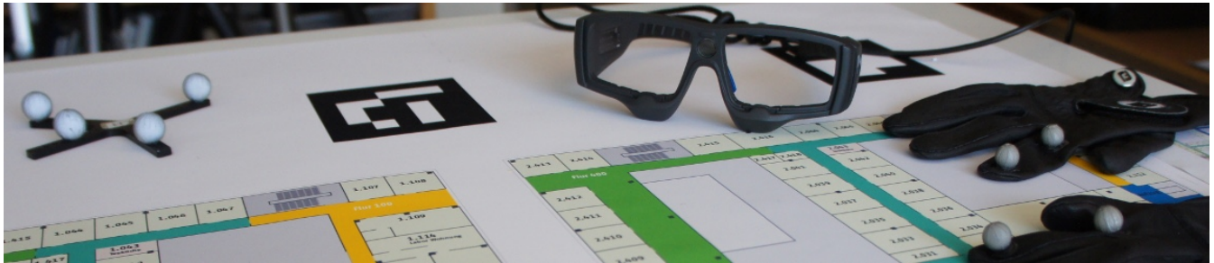
Figure 1: The scenario: The task is to plan routes on floor plans of a larger building. Human communicative behaviour including gaze and gestures are recorded using mobile eye tracking glasses and gloves with optical marker tracking.
