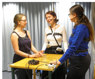
Figure 1: Recording setup. The white boxes are earlier prototypes of our respiratory belt processors.
