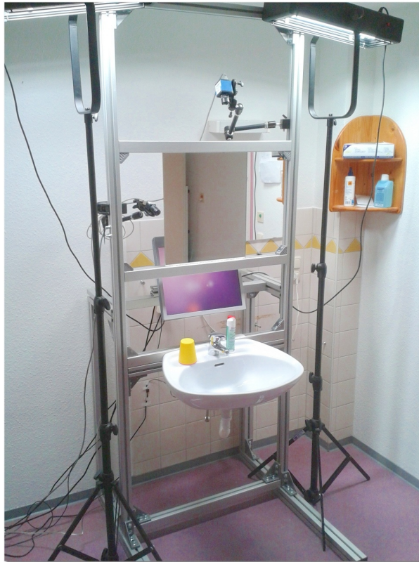
Figure 4: Washstand setup equipped with sensor technology.
