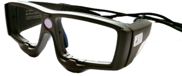
Fig. 5. SMI Eye Tracking Glasses, a binocular mobile eye tracker.
