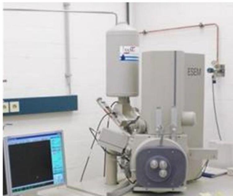
**Figure 2.6** On the top the schematic representation [75] and at the bottom picture of the SEM setup imaging of samples with a relative humidity of up to 100% under low-vacuum conditions.
