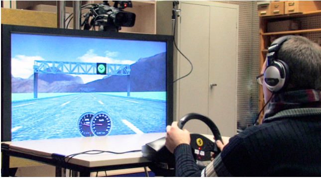
Figure 4. Example of task: user is seated in front of steering wheel and a large screen, the speech is presented via the headphones.
