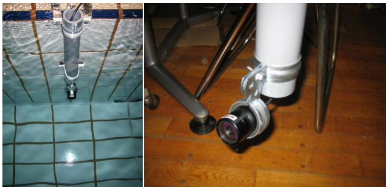
Fig. 1 Custom made fixed tools with under water CCD cameras.
