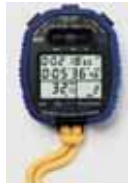
Fig. 1 A race stop watch specialised to measure simultaneously time and the stroke rate per minute (N) – here N = 32 / \text{min} .
