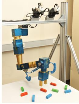
Figure 1.1.: Robotic agent for the study of object interactions consisting of a stereo camera head (2 DOF per camera) and a robotic manipulator (6 DOF) with attached two-finger gripper.
