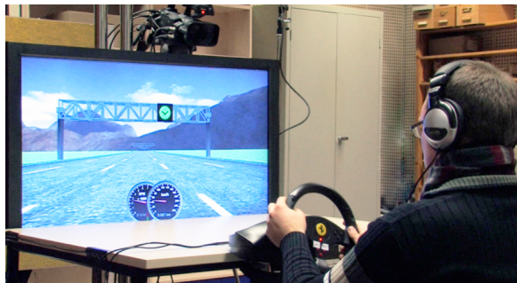
Figure 3: View of experiment setup: a driving simulation, interfaced with a steering wheel and pedal, is shown on the large screen. Speech is presented to the participant via headphones
