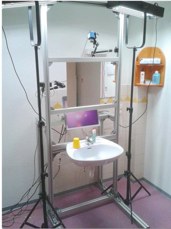
Fig. 2. Washstand setup equipped with sensor technology.
