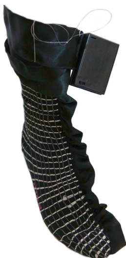
Figure 2.4: Pressure sensitive sock Smart Sock [Sma] by Alpha-Fit GmbH. (Photograph taken with the permission of booth personnel during a visit to the Medica Fair 2013)
