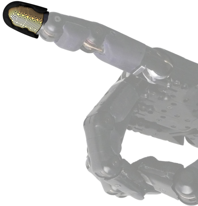
Figure 4.8: Resistive fingertip tactile sensor with an anthropomorphic 3D shape with 12 tactile cells and embedded signal processing electronics for a human sized dexterous robotic hand. (Note that the cutout in the sensor material covering the electrodes is for illustration purposes only.)
