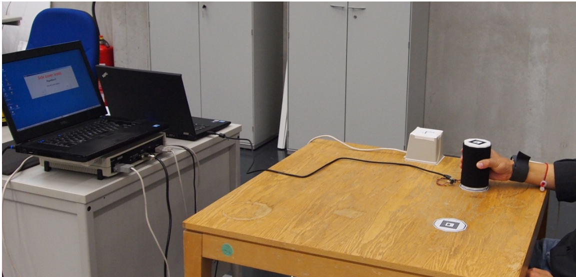
Figure 3.48: Experimental setup for grasp quality metrics evaluation. iObject was picked up and placed down by participants between two predefined positions on the table using a grasp type and pace according to presented visual and audio stimuli.
