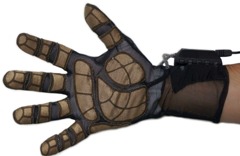
Figure 3.15: Second prototype of a wearable right hand dataglove with 54 taxels and embedded data acquisition electronics.
