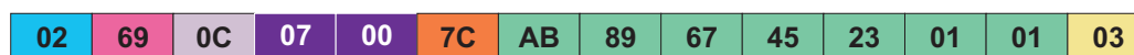
(b) An example of incoming link notification packet when connected from Bluetooth host 01:23:45:67:89:AB. The local RFCOMM port chosen in iObject will always be 0x01 .
