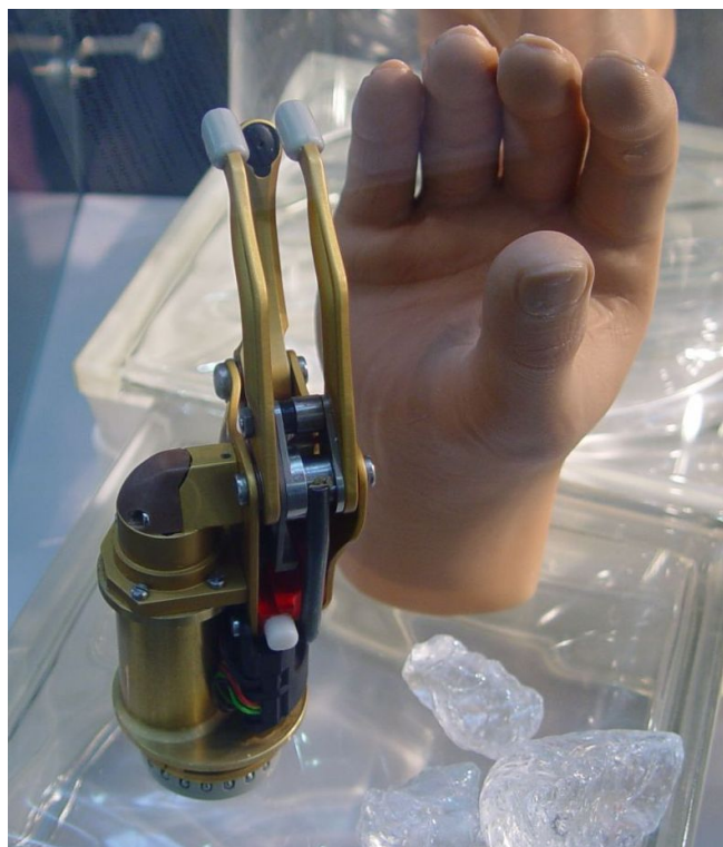
Figure 2.7: Single degree-of-freedom hand prosthesis. (Photograph taken with permission of booth personnel during a visit to the Hannover Fair 2006.)
