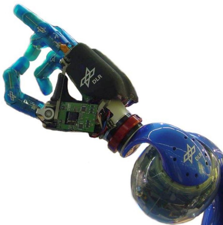
Figure 2.10: DLR-Hand II with integrated 6D force/torque sensors located in each fingertip [BGLH01]. (Photograph taken with permission from booth personnel during visit of Hannover Fair 2004.)
