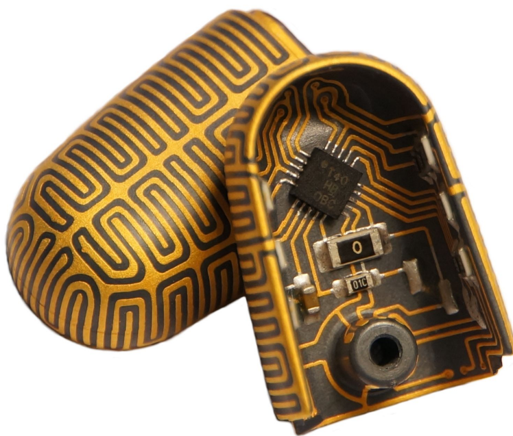
Figure 4.15: Finished fingertip electrode prototypes displaying the soldered data acquisition electronics embedded on the inside of the MID.
