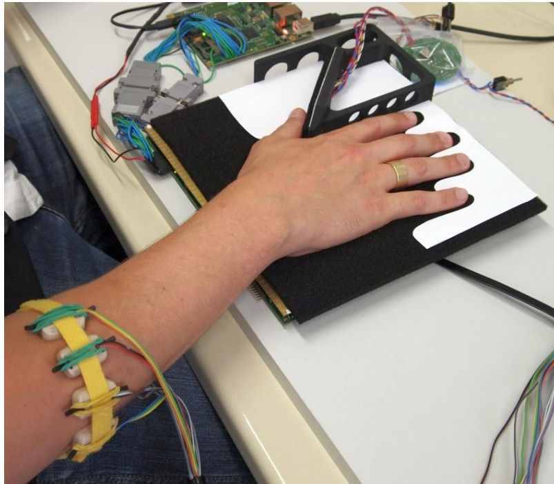
Figure 3.52: An experimental setup to capture the mapping of single finger forces to muscle activations using sEMG electrodes around the forearm and tactile sensor array below palm and fingers for force measurements.
