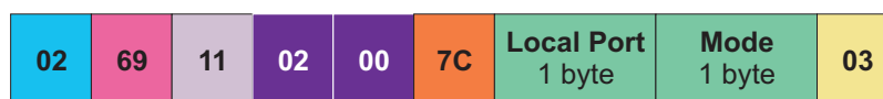
(a) SPP_TRANSPARENT_MODE packet. When leaving the transparent mode, the Mode field will be set to 0x00 .
