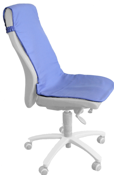
Figure 3.1: A version of tacTiles touch sensitive mat to cover an office chair.
