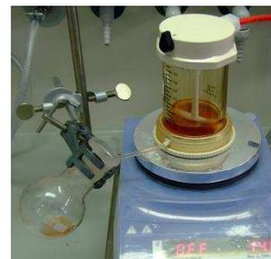
**Figure 54.** Stirring cell with ultrafiltration membrane for the removal of dissolved  $\alpha$ -chymotrypsin after the desymmetrization reaction.
