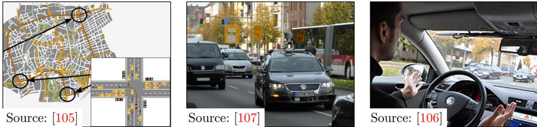
Figure 2.3: The autonomous vehicle *Leonie* of the Braunschweig *Stadtpilot* project is capable of driving in real-world urban traffic, but requires laser-based and radar-based perception with GPS information instead of visual sensors.
