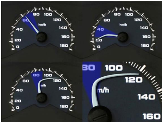
Figure 5. Curvy Speedometer [29]. The tip of the needle indicates the current speed of the car while its curvature indicates, how far the current speed is from the most fuel-efficient speed
