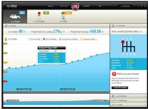
Figure 4: Screenshot of the Fiat eco:drive software [13]. The software uses data that was captured while in the car and assesses various aspects of driving behavior.
