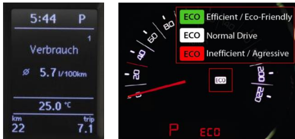
Figure 2: (a) Basic display of instantaneous fuel consumption, measured in L/100km [8]. (b) Eco-driving indicator, which is integrated into the speedometer and can differentiate between three levels of fuel economy [6].
