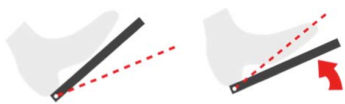
Figure 3: Active acceleration pedal (Eco Pedal). When pressing the pedal beyond the dotted red line, the pedal actively exerts counter-pressure [10].
