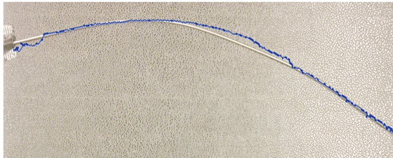
Figure 6.34: The tracking result (blue) superimposed on the actual cable. Despite a slight overshooting, the cable is tracked very accurately.
