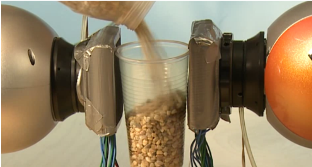
Figure 6.30: Using the slip detection and grasp force adaption, two robot fingers equipped with Myrmex modules can master dynamic scenarios. They hold a plastic cup (2g weight) while it gets filled with 250g of small stones.
