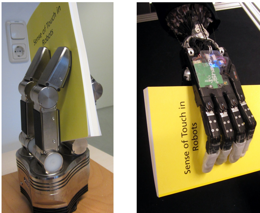
Figure 6.2: Left: The Schunk SDH hand with three fingers is a robust hand that is also used in industrial applications. Right: The anthropomorphic Shadow hand with five fingers has a dexterity that is comparable to humans. [103]
