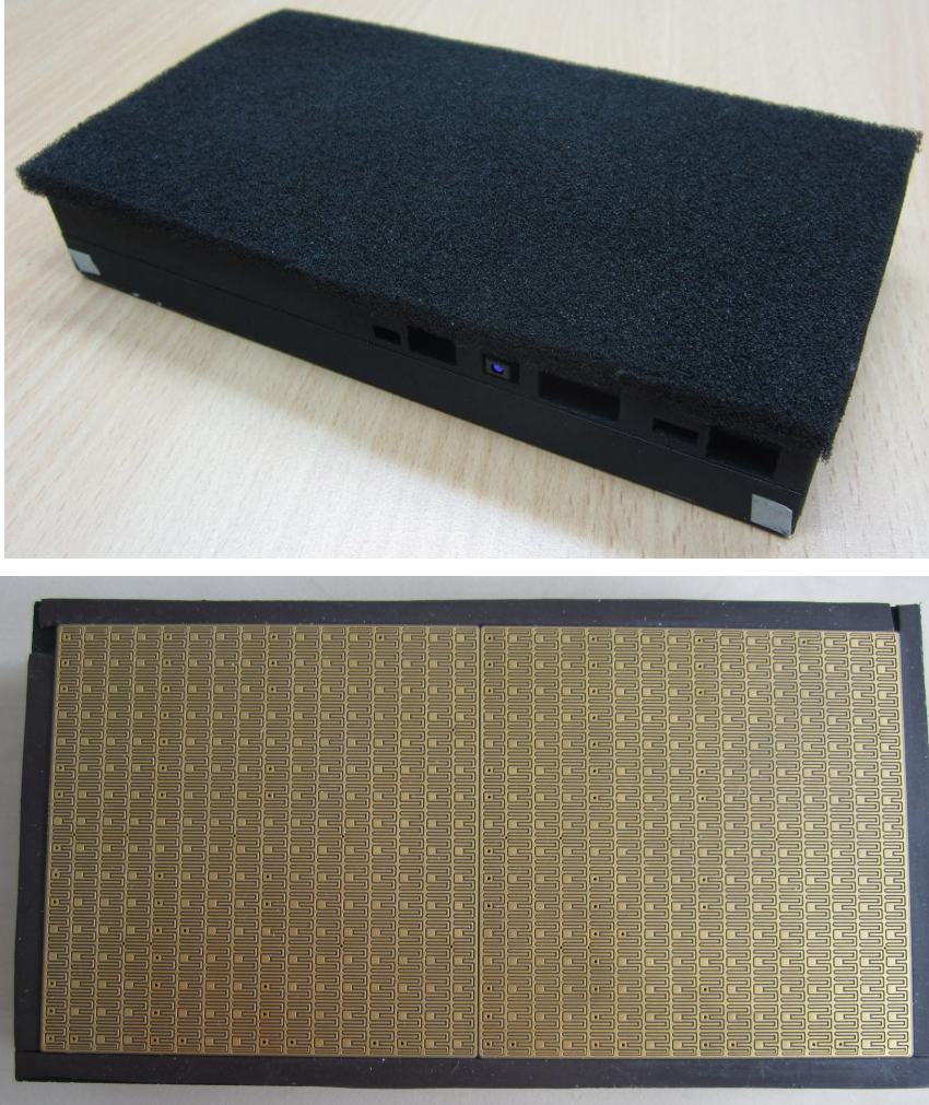
Figure 4.3: Top: The Myrmex tactile book in cable free operation mode. Like the other Myrmex modules, it needs to be covered with a conductive elastomer to allow the tactile sensing capability. In this case a black polyurethane foam is used. Bottom: The top side of the tactile book without the elastomer. One can see the sensor surface of two Myrmex modules. The tactile surface is surrounded by adhesive magnetic strips attached to the edges of the book. The foam cover is equipped with the same strips, which allows for an easy and secure attachment of the foam to the book.
