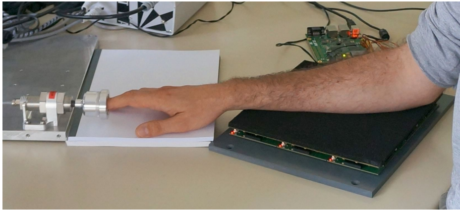
Figure 6.26: The experiment to develop a tactile based prosthesis control. This time the forearm is placed on the Myrmex table and the fingers are placed in a force sensing device. The tactile profile of the forearm (visible on the screen) is then correlated to the exerted finger force.
