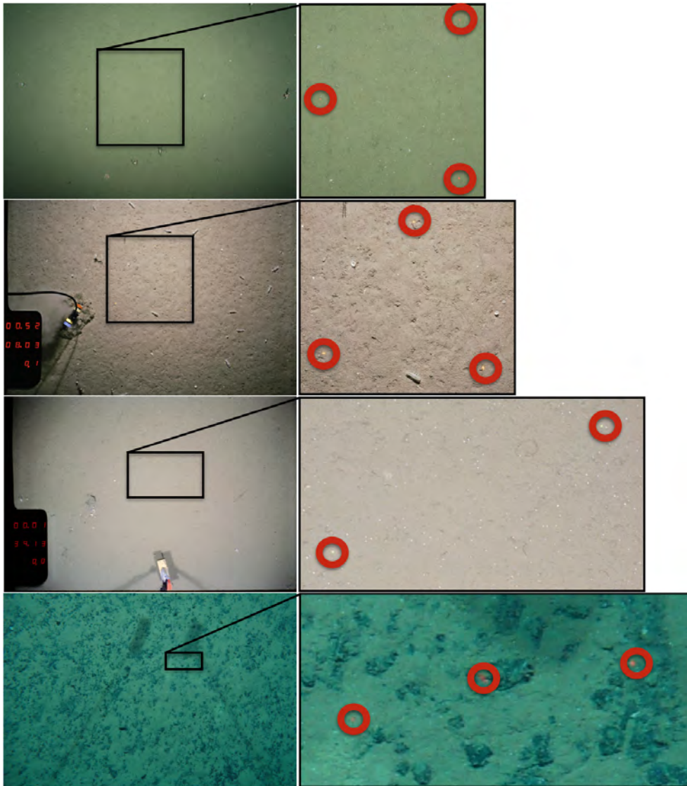
Figure 6.2: Four examples of different LP spatial layouts. The left column shows the full images as they are acquired. The black box highlights the region within the image in which the LPs are visible. Those parts are cropped out and magnified (right column) and the occurring LPs are marked by red circles. The third row shows the case of a two-LP layout.
