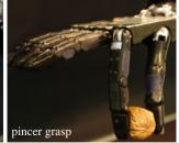
**Fig. 2** Three basic grasp prototypes used for the Shadow Dexterous Hand. Depending on object size, estimated weight, and envisioned manipulation task we choose from a power grasp, a precision grasp, and a pincer grasp (*left* to *right*)
