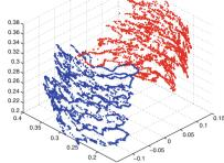
**Fig. 11** Tactile object exploration using two tactile sensor arrays mounted onto Kuka LWR arms (*left*) and the resulting tactile point cloud as a local estimation of object shape (*right*)
