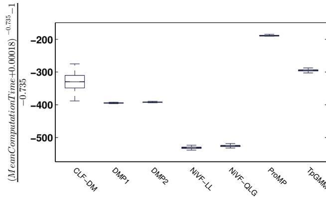
Fig. 4.5: Results of the benchmark comparing five different models over all shapes and benchmark conditions showing the mean computational time during the benchmark tests.
