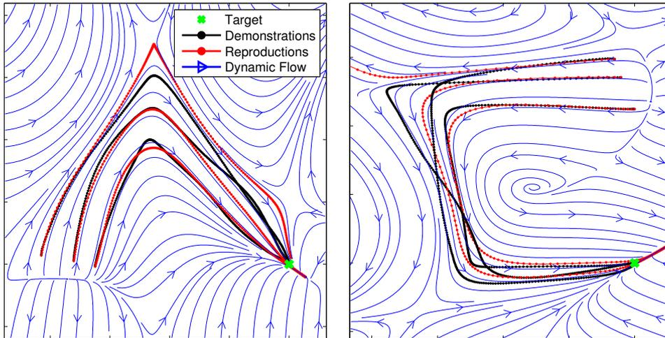
Fig. 3.3: Unstable estimation of dynamical systems through demonstrations. Data were taken from the LASA dataset: A-shape (left) and sharp-C (right). Note that the reproduced trajectories either diverge or converge to spurious attractors.
