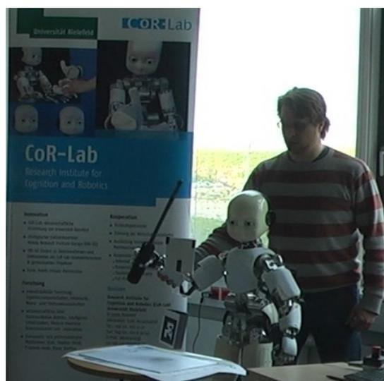
Fig. 8.6: Kinesthetic teaching of the fishing motion skill with iCub. iCub holds a fishing rod in its right hand and tracks the marker at the fishing hook by moving his head. The fish is indicated with a marker for visual tracking. The fishing hook is also static in orientation.
