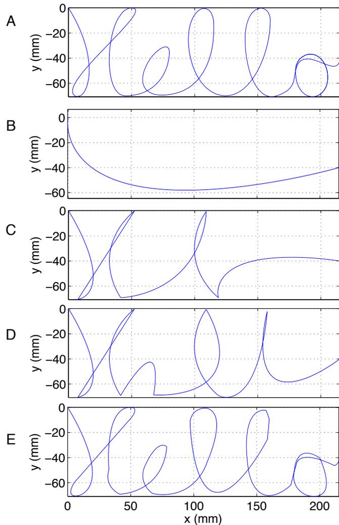
Fig. 7.9: Decomposition of the word “Hello” with different settings. (A) Final decomposition with Eq. (7.3) as matching criterion (area between trajectories). (B) Final decomposition with Eq. (7.1) (maximum error). (C) Final decomposition with Eq. (7.2) and precision  $p = 20$ . The decompositions are slightly different in each case, however, the capability of decomposing and representing the demonstration appear robust with respect to different matching criteria and precision of primitives.
