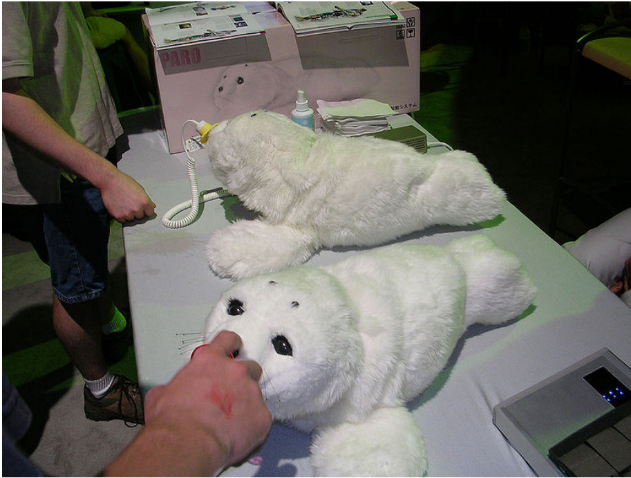
Figure 2.1.: The robotic seal paro designed by the Intelligent System Research Institute of Japan's AIST. The robot is used in long-term interaction with elderly people in health care facilities.
