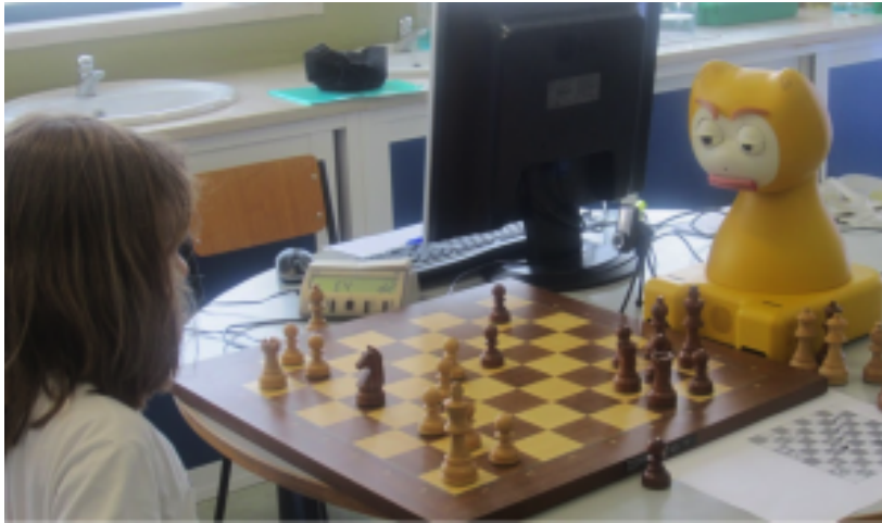
Figure 2.3.: The robot iCat. In the scenario the robot plays the game chess with participants. The robot advises the player on the turns to be played.
