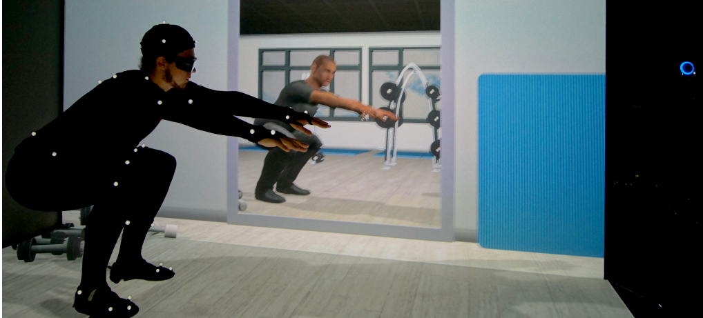
Figure 1: Real-time feedback using a virtual mirror requires an immersive Virtual Reality environment that provides full-body motion capturing, motion analysis, and realistic character rendering at a low end-to-end latency.
