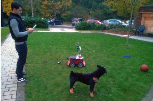
Fig. 5. Typical scene of the interactive scenario. The robot drives randomly on the grass area and encounters various objects. The user follows the image-stream on the iPad and can label approached objects.
