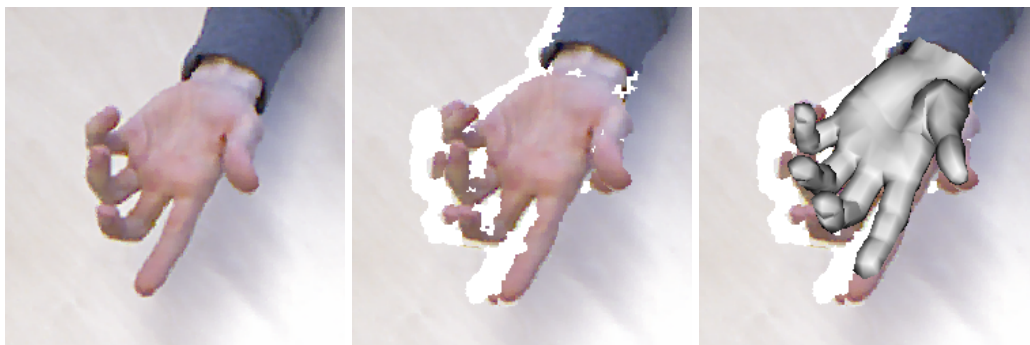
Figure 5.1: The user’s hand posture is estimated in real-time by fitting a 3D hand model to the Kinect point cloud using inverse kinematics.
