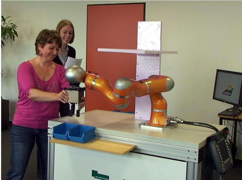
Fig. 4.8: Participant of the FlexIRob@Harting study during the *CONFIGURATION* phase teaching the LWR IV redundancy redundancy resolutions in the second training area of the confined workspace.
