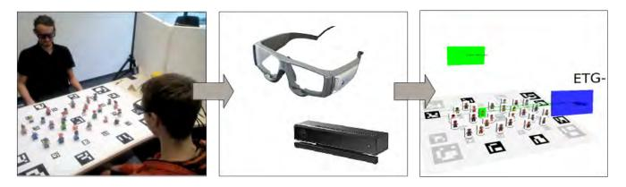
**Figure 3:** EyeSee3D process: left: real world figure identification task; middle: interaction is tracked using different sensors, such as eye tracker or Microsoft Kinect; right: EyeSee3D fuses tracking data in a 3D situation model including areas of interest for all figures and the heads of the interaction partners (boxes). The picture shows a screenshot from the EyeSee3D preview window for the situation at the left.
