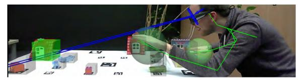
**Figure 1:** EyeSee3D analyses eye gaze on dynamic areas of interest in 3D environments. Objects and body parts can be tracked using a variety of tracking systems. Data is fused in a common 3D situation model. The example shows tracked head, hands, and gaze, as well as target stimuli of a LEGO toy kit. The user's gaze (blue) currently fixates a part of the roof (highlighted in green on the left).
