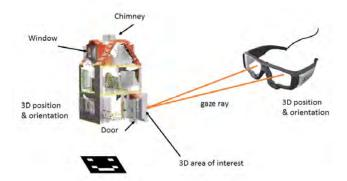
**Figure 2:** A 3D situation model is used to determine the objects of interest the user is currently fixating on. In this example, printed fiducial markers are used to create a common coordinate frame in which the eye-tracking system and the target objects are represented.
