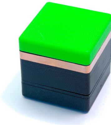
**Figure 7.4:** The touch sensing enabled TAO. A band of copper was wrapped around the upper part of the TAOs' housings, acting as the antenna.
