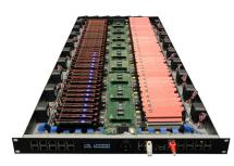
Figure 2: Example of a RCU, equipped with 72 **ARM** compute boards
