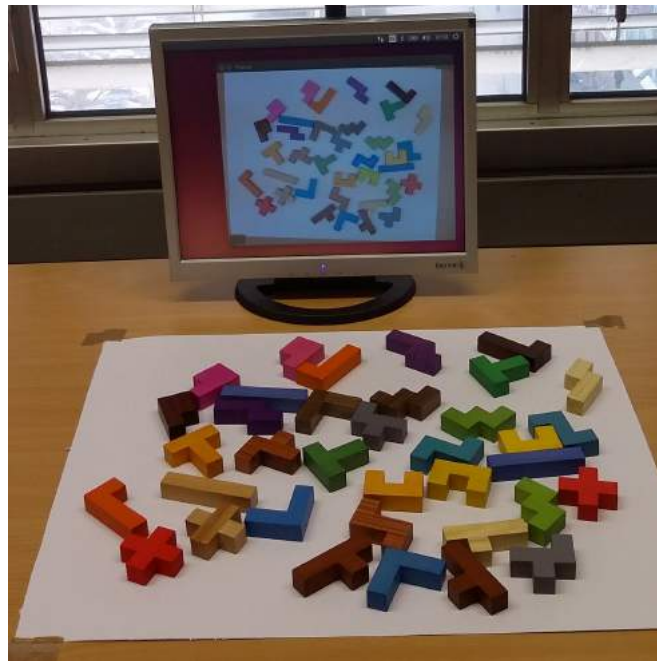
Figure 4.7: Depiction of the TAKE-CV task; the participant sat at a table with 36 PENTO objects. A camera (not pictured, though the feed the camera produced can be seen in the screen behind the objects) fed the image information to the computer-vision software which randomly picked which object to select as the referent, and (if applicable) as the landmark. Those selections were displayed on the screen behind the objects.
