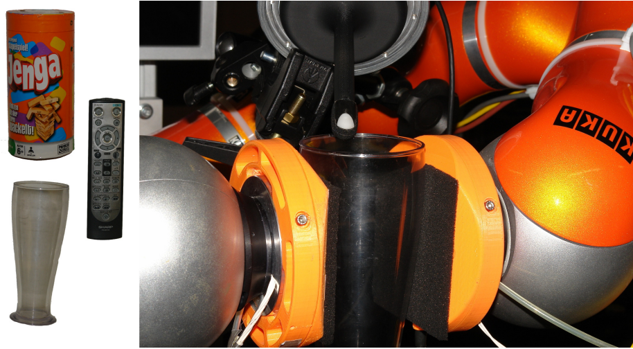
Fig. 1: Objects used for the evaluation and experimental setup for data recording. Two KuKa LWR robots with attached tactile sensors (light orange) holding a glass. The fingertip shaped sensor touching the glass from above is used to detect the onset of slippage for data labeling purposes.
