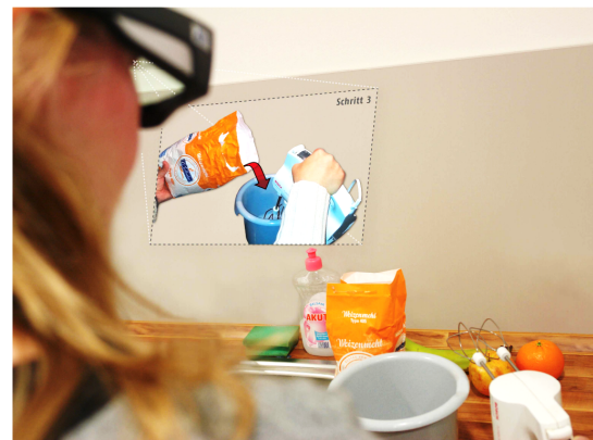
Figure 1: ADAMAAS will provide situation-, user-, and action-specific feedback on a transparent virtual plane superimposed on the user's field of view.
