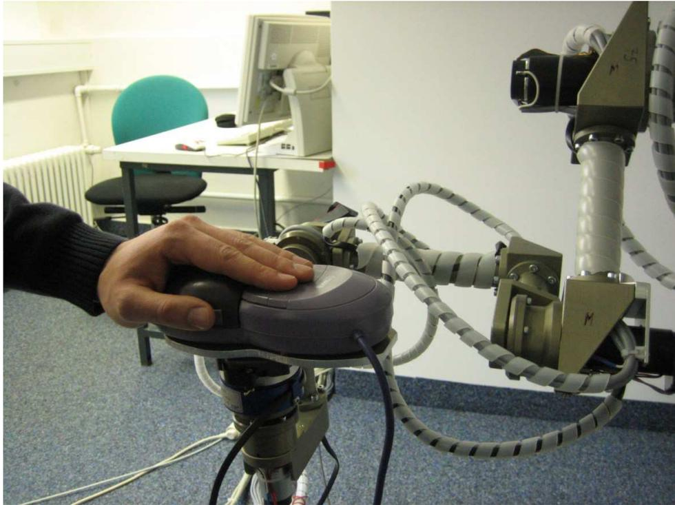
**Figure 4.8:** VirTouch Mouse mounted on ViSHaRD 10.
