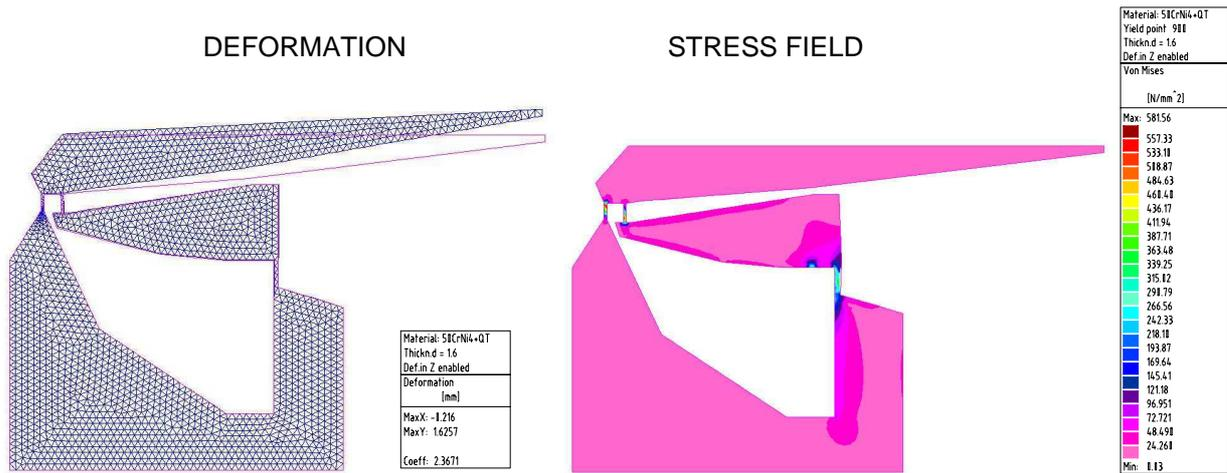
**Figure 2.9:** Final FEM design loop of the combined lever system
