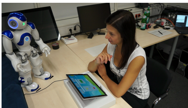
Figure 2: Experimental setup (left) with a participant sitting in front of a tablet displaying the graphical user interface (right). The robot Nao stands next to the tablet slightly rotated towards the user.
