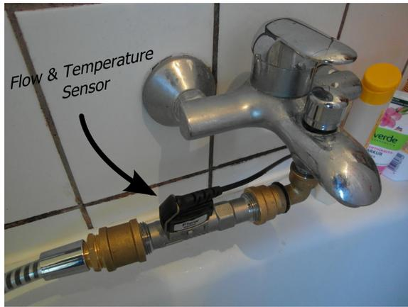
Figure 2: Picture of the flow sensor used in the InfoDrops setup.
