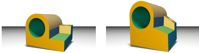
Figure 8.10: Deformation of the Joint model using automatically detected geometric primitives. Left: Original setup keeping the bottom fixed and using the top cylinder region (golden) as a handle. Right: Deformed model.
