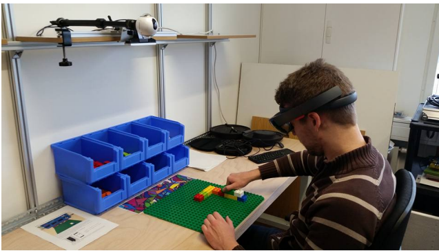
Figure 3: HoloLens smart glasses providing in-situ AR assistance
