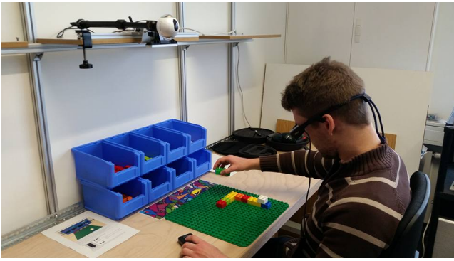
Figure 5: Moverio BT-200 smart glasses showing central in-view pictorial instructions
