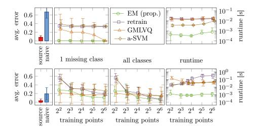
Figure 2: Average classification error (left) and runtimes (right) for the artificial data set (top) as well as the myoelectric data set (bottom). We show the number of available target space training data points on the x axis (in log scaling) and the average classification error (linear scale) and runtime (log scale) respectively on the y axis. The standard deviation across trials is marked by error bars.
