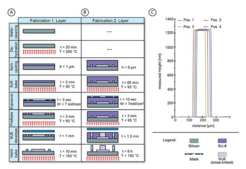
**Figure 3. Illustration of two layer wafer fabrication process.** (**A**) Fabrication of the first layer containing trapping structures; (**B**) Fabrication of the second layer containing fluid channels, inlets and outlets; (**C**) Representative surface profiles of the first layer. In this case the height of the first layer was 1,200 nm and is used for the cultivation of *C. glutamicum* in complex medium.
