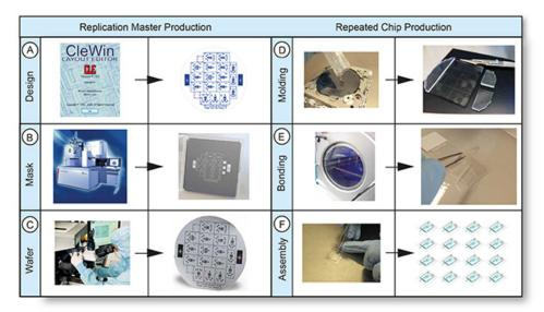
**Figure 1. Overview of PLBR chip production process.** Master mold fabrication: starting with (**A**) Design, (**B**) Lithography mask fabrication, and (**C**) Wafer production. PDMS-glass chip production: starting with (**D**) of PDMS molding followed by (**E**) glass and PDMS bonding and (**F**) final chip assembly.
