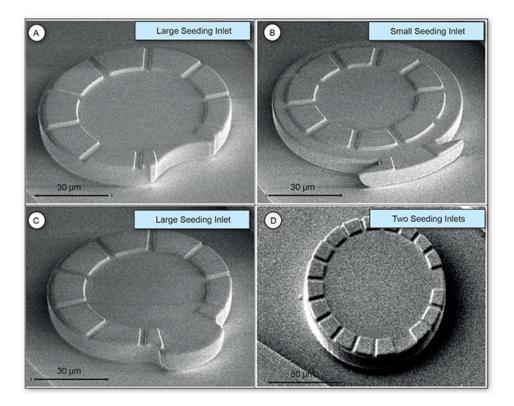
**Figure 8. Scanning electron images of different PLBRs.** SEM images showing seeding inlets for the optimization of trapping efficiency. (**A**) Lager seeding inlets (**B**) Smaller seeding inlets (**C**) Larger "open" seeding inlets (**D**) Two seeding inlets.
