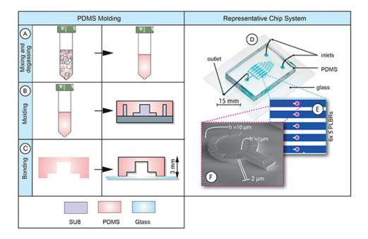
**Figure 4. Device fabrication and representative chip.** Illustration of the PDMS molding process: **(A)** PDMS mixing and degassing; **(B)** PDMS molding; **(C)** mold release, cutting and chip bonding. Final chip (Reproduced with permission of the Royal Society of Chemistry <sup>13</sup>): **(D)** photograph of the PDMS chip with 2 inlets and 1 outlet; **(E)** CAD image of six parallel arrays containing 5 PLBRs each; **(F)** SEM image of one PLBR.
